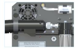
Please note that the mechanical is connection is obtained thru a quick coupling connector. In order to attach the probe, it's sufficient to push it in, and lock the probe with the dedicated bracket (with 4x M4 screws) to the back of the device.
